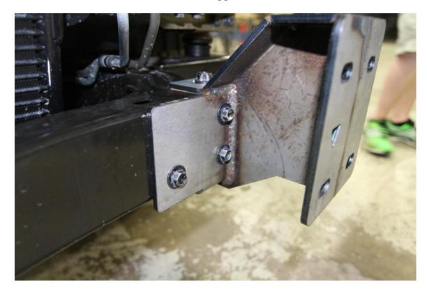
B. Mount bumper to bracket. With the help of at least two others and possibly a floor jack, to support the center of the bumper, lift the Fab Fours bumper into place. <u>Do Not</u> <u>Fully Tighten, Hand Tighten Only.</u>
