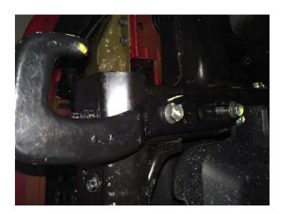
7. Remove the bumper mount brackets from both frame rails using a 14mm socket. Save this hardware for later use.
