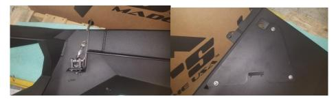
**3.** While the fender is on the floor, install the marker lights and grommets to the fender. Run the wires along the zip tie holes and through the internal hole in the fender. Allow the marker light wires to hang into the wheel well opening.
