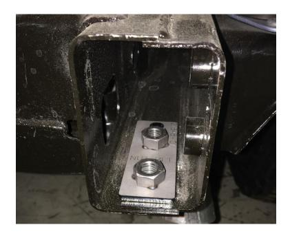
13. With a friend, carefully hold the bumper and swing arm assembly up to the Jeep and use the ½" bolts to attach the nut plate along with the OEM side bolts.
