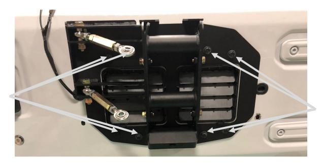
6. Take the rubber stops and attach them to the swing arm using the 3/8" bolts. (Make sure to push the stops up against the metal gussets as shown before fastening)
