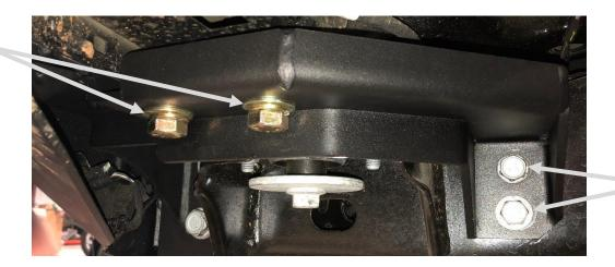
15. Take the turn buckles and put them through the swing arm and attach them using the ½" bolts with spacers and washers. (Tighten securely)
