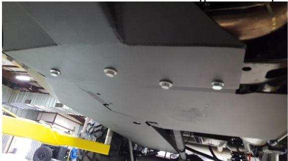
**4.** Using the provided 7/16" hardware, attach the brackets to the vehicle's engine mounts. The driver's side bracket will pick up the rear slot. The passenger's side bracket will pick up the front slot.
