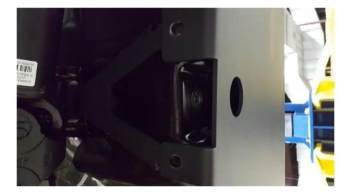
**5.** Remove the rear inner bolt on the gas tank using an 18mm socket and loosely attach the bracket by replacing the bolt. Attach this bracket to the skid plate.
