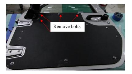
3. Once bolts are removed, use the provided hardware to install the mirror guard reusing the existing top four mounting locations of the skin. Using the provided hex head bolt in the location closest to the door handle.
