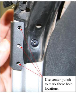
2. Next using a 9.00mm drill bit ("T" size drill bit will also work) drill the marked holes. Some of the holes will have to go through 2 layers. See image below.
