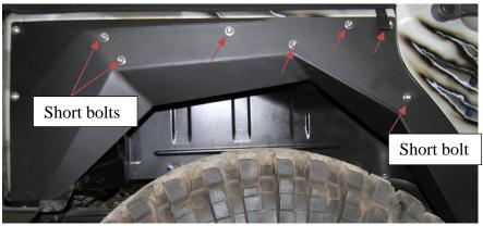
2. <u>Next place fender flare on fender</u>, lining up mounting holes. Start by re-installing the three short bolts to hold flare in place.
