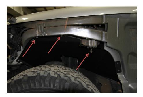
**3.** Mark the three lower mounting points in preparation for drilling the piolet holes.
