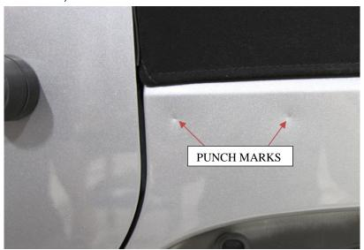
**4.** Once fender is removed, you can begin drilling. Start out by drilling all punch marks with the  $\frac{1}{4}$ " drill bit. Follow behind that with the  $\frac{1}{3}$ " drill bit.
