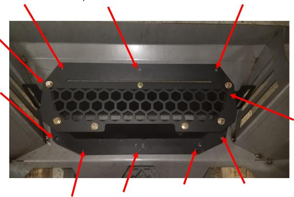
**3.** Install mesh to back of light box with the supplied 5/16 hardware.
