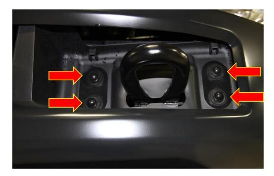
2. Next, with the help of someone holding the bumper in place, remove the four 15mm bolts from the bumper supports on both sides of vehicle.
