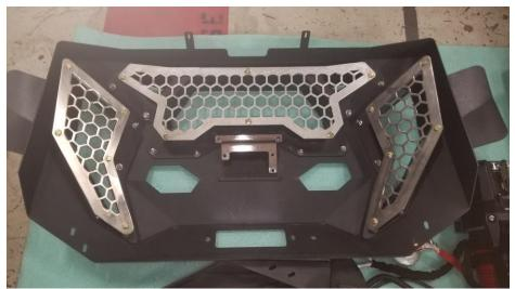
3. If installing an Adaptive cruise control module install module to the included bracket using the provide M8 nuts. Then install bracket to grill section using the 2 lower center insert 5/16<sup>°</sup> bolts
