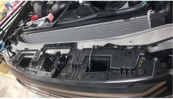
8. If equipped with front camera remove the camera washer Tee from the main washer line and reconnect the main washer line to itself the can be done by pulling up on the black retainer collar.
