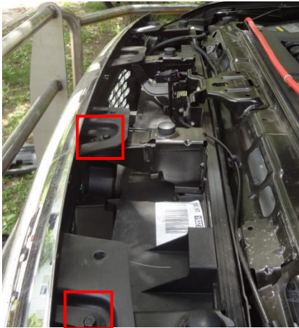
Figure 2a-bolts on LH side
