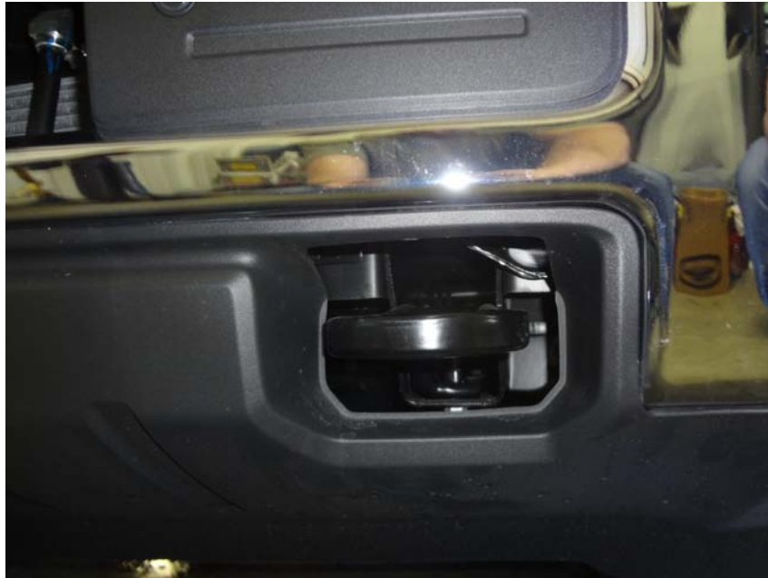
Figure 1a (TOW HOOK HOLE W/ OEM TOW HOOK)
