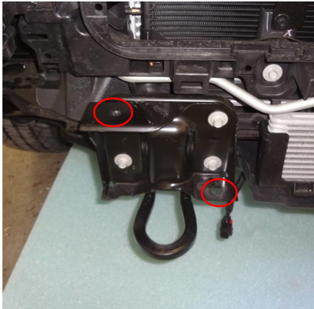
Figure 3a (TOW HOOK & OEM MOUNTING BRACKET)
