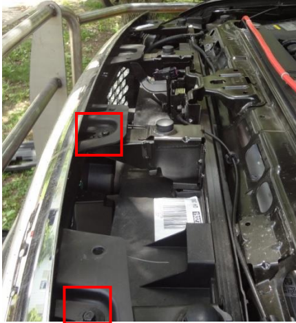
Figure 2a-bolts on LH side
