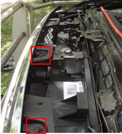
Figure 2a-bolts on LH side
