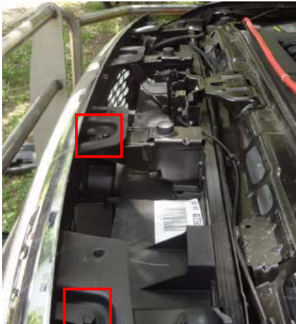
Figure 2a-bolts on LH side
