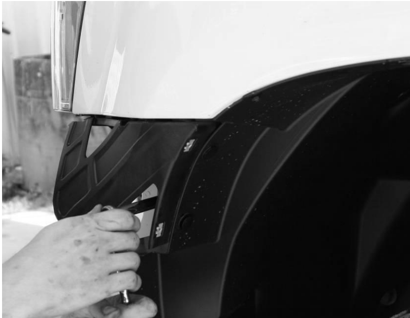
Figure 6 - Support Bracket Removal
