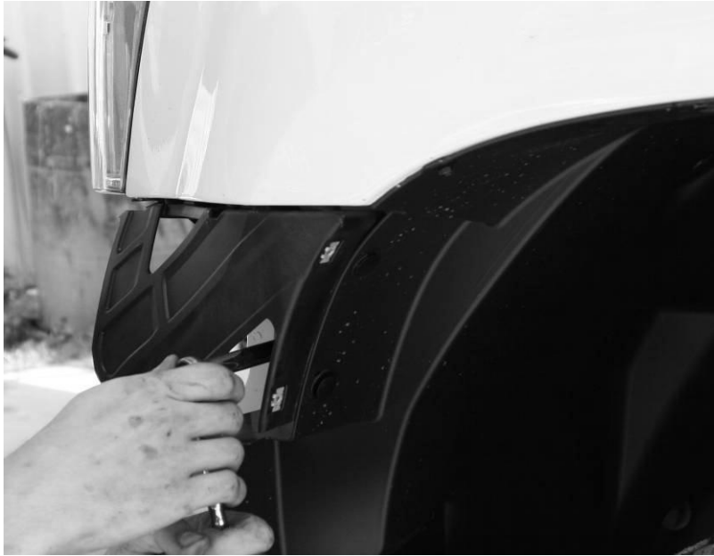
Figure 6 - Support Bracket Removal
