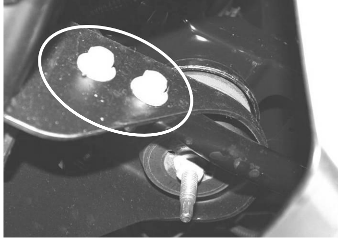
Figure 4 – Outer Bumper Support Screws
