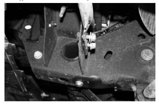
7. Remove the dart clips holding the rubber valence between the frame and the bumper.
