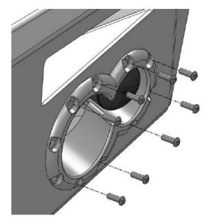
G. Install the Fab Fours fog lights onto the mounting brackets as shown below using the #8 button head screws, washers, and hex nuts.
