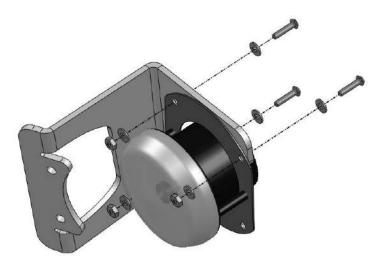
H. Install the fog light and bracket into the bumper using the remaining two holes available in the light insert. Use the 1-1/2" length <sup>1</sup>/<sub>4</sub>" stainless steel button heads with <sup>1</sup>/<sub>4</sub>" washers and nuts.
