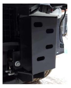
B. Install the provided stud plates from inside the winch tray with the threads pointing to the rear of the vehicle. Secure with retaining washers.
