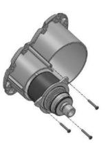
F. Install the light inserts with turn indicators into the cutout in the bumper. Use the <sup>3</sup>/<sub>4</sub>" length <sup>1</sup>/<sub>4</sub>" stainless steel button head, <sup>1</sup>/<sub>4</sub>" washers and hex nuts to fasten the insert through the holes shown below:
