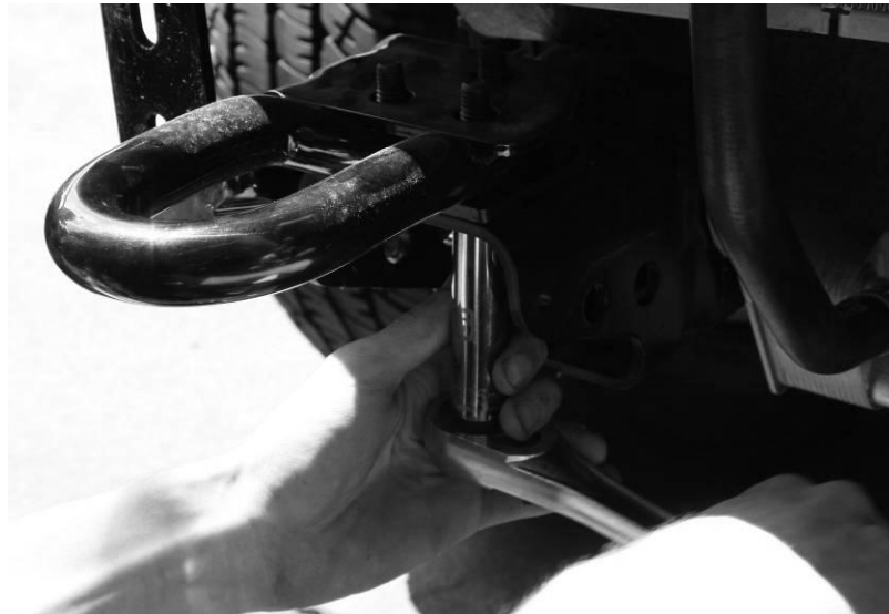
Figure 3 - Tow Hook Removal
