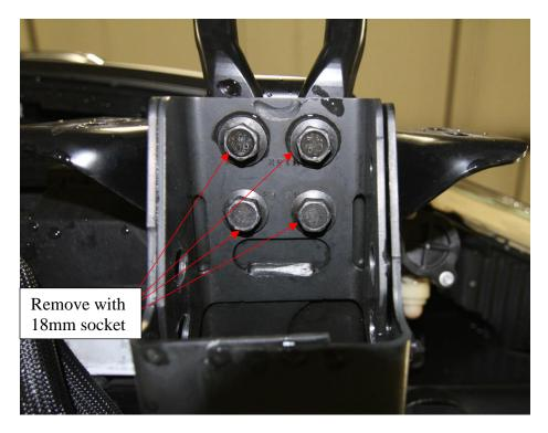
5. Next using 18mm socket remove the two nuts on either side of the frame attaching frame horns to frame. Set bolt strips and nuts aside as they will be used in the installation of Fab Fours bumper. (See image)
