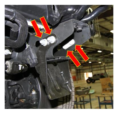
6. With the bumper lying face down, begin removing the inner structure of OEM bumper. Start by removing 10 bolts using 8mm socket.
