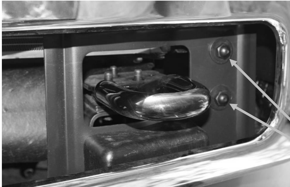
Figure 1 - Bumper Mount Bolts
