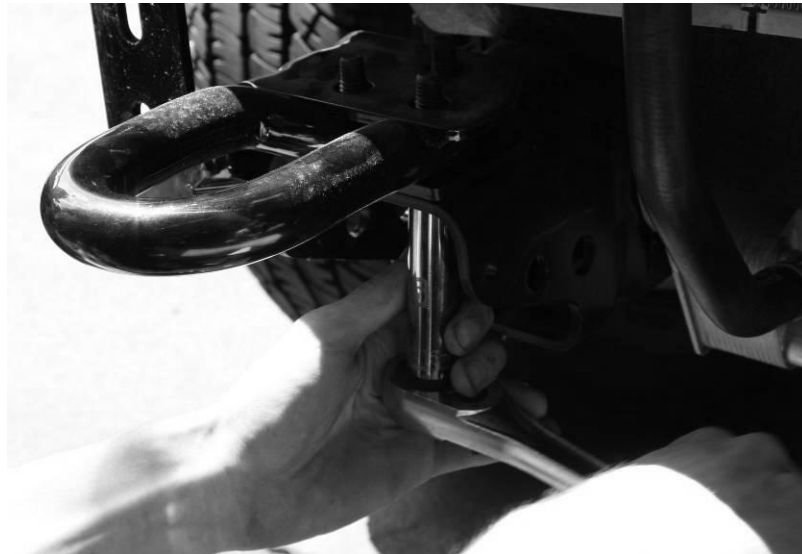
Figure 3 - Tow Hook Removal
