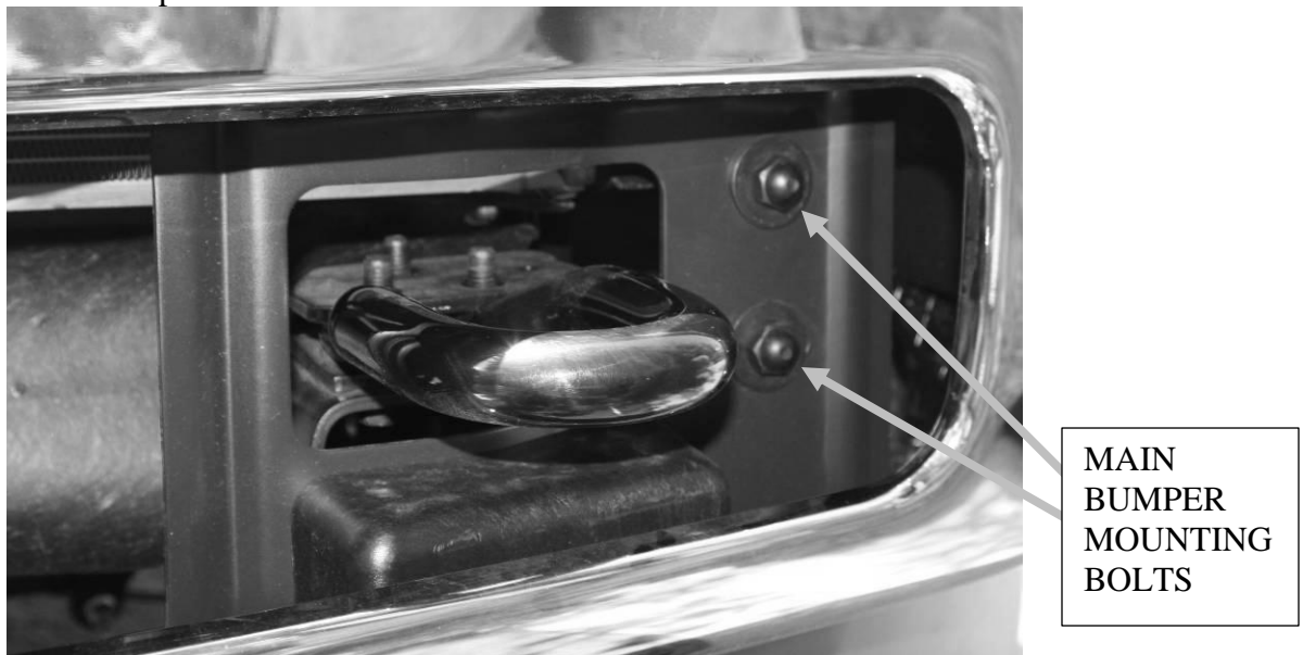
Figure 1 - Bumper Mount Bolts
