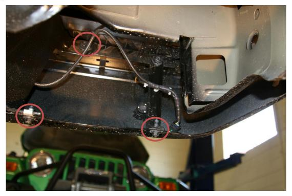
E. Using two people each grasping one corner of the bumper lift and rotate towards the back of the vehicle. Note the are two plastic locating finger that pass through the hitch that need to be freed for the bumper to come off.
