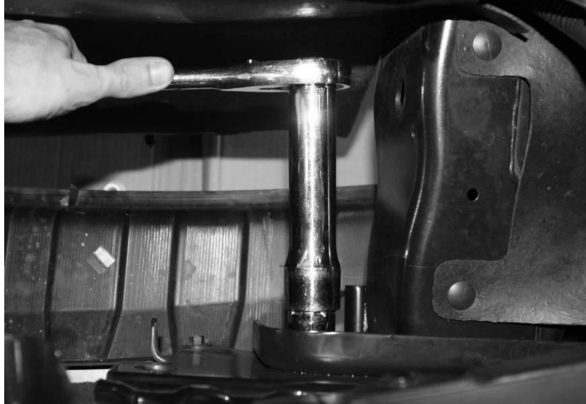
Figure 2 - BUMPER MOUNTING BOLTS (VIEW FROM TOP)
