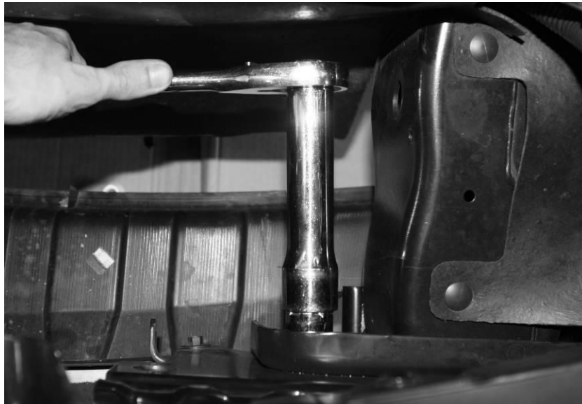
Figure 2 - BUMPER MOUNTING BOLTS (VIEW FROM TOP)
