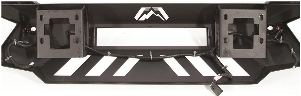
Figure 9a (OVERALL SENSOR HARNESS ROUTING)
