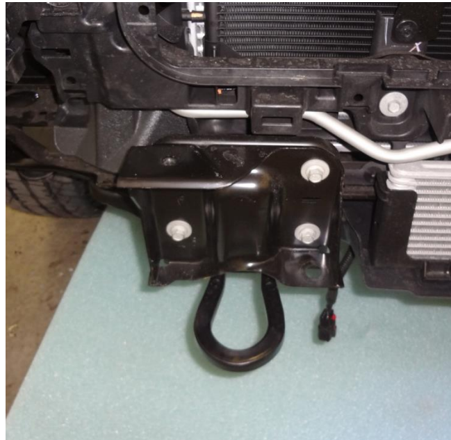
Figure 3b (TOW HOOK & OEM MOUNTING BRACKET)
