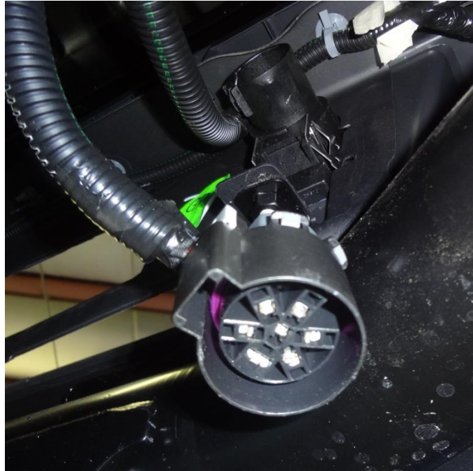
Figure 3a (ELECTRICAL HARNESS DISCONNECTED)
