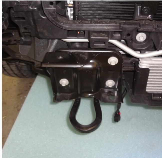
Figure 3b (TOW HOOK & OEM MOUNTING BRACKET)
