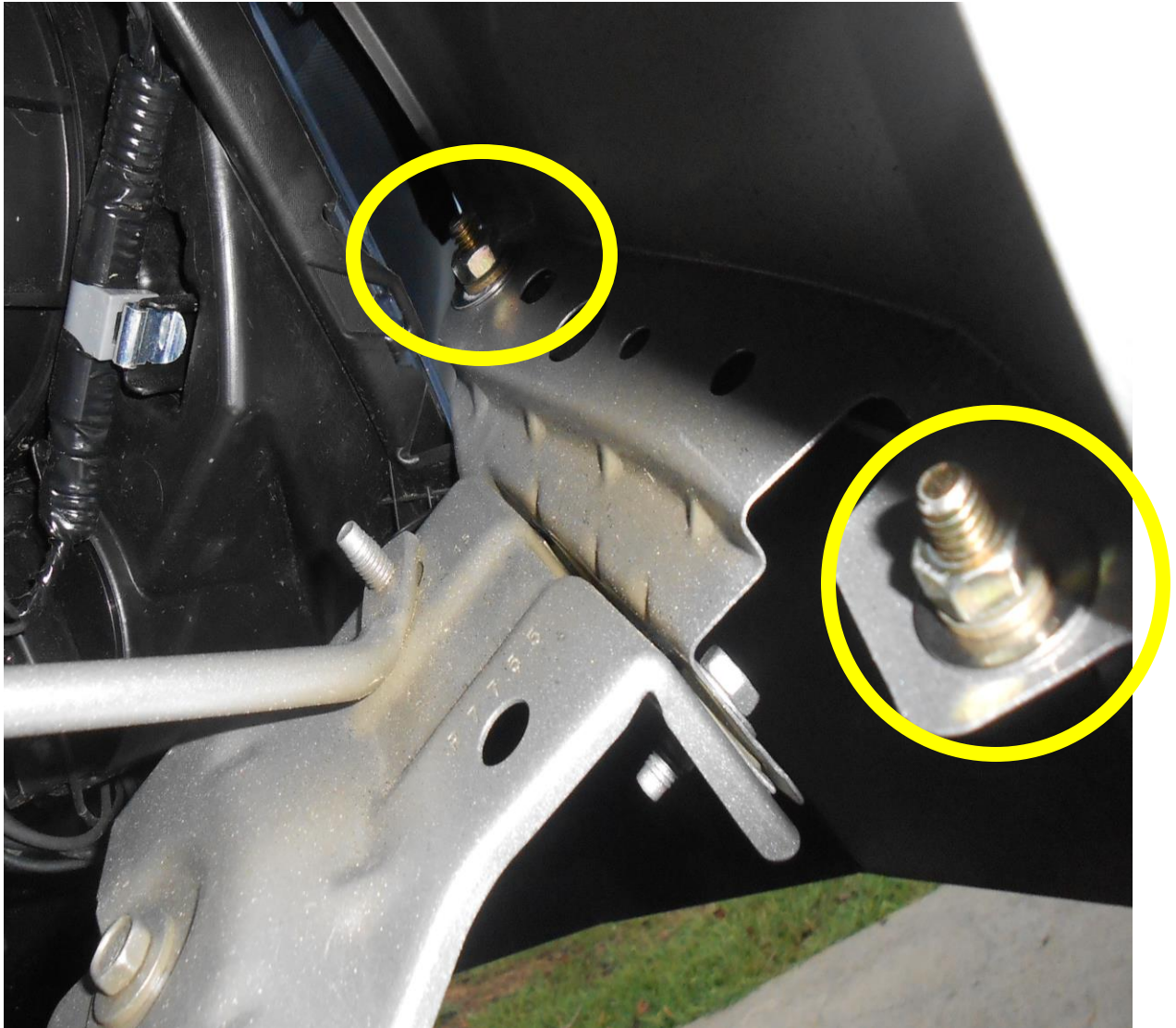
Figure 6b (bolts through mount points on fender)
