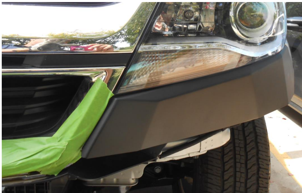
Figure 5c (valence position relative to grill)
