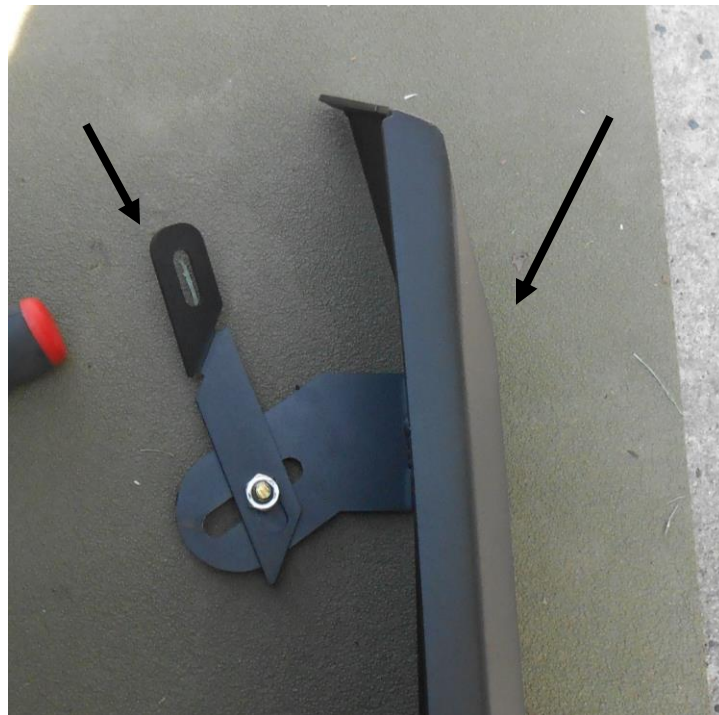
Figure 5a (valence loosely bolted to valence mount)
