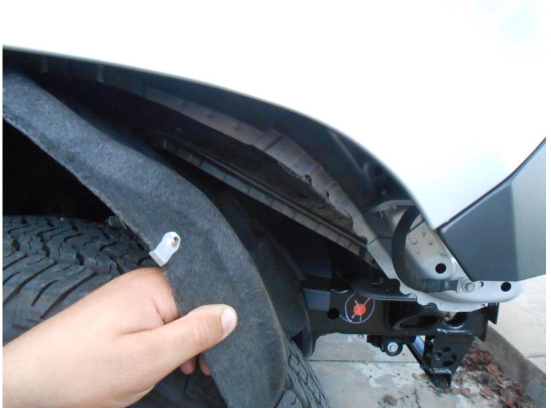
Figure 6a (wheel well liner pull back)
