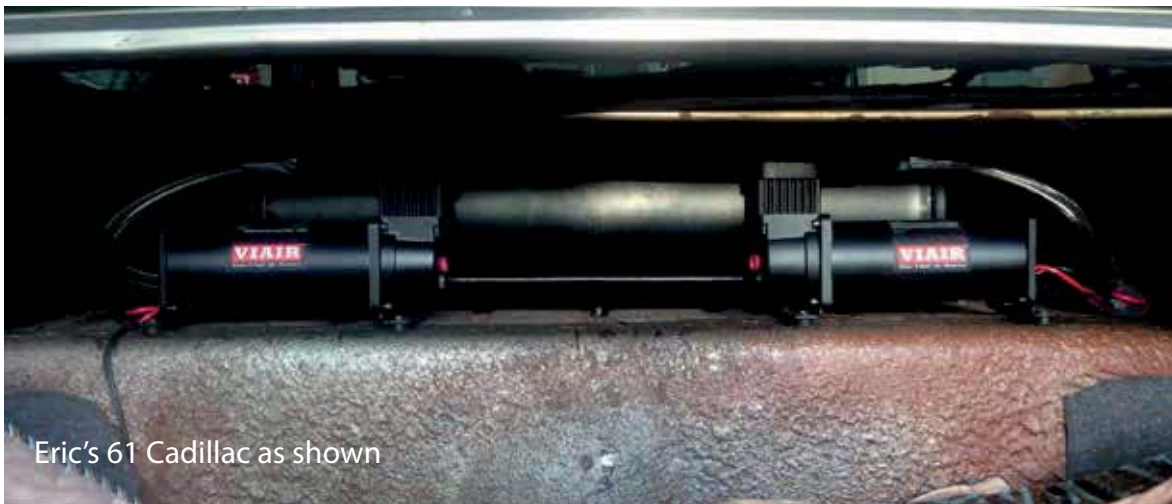
In tight spaces use washers to adjust tank height, as shown.
