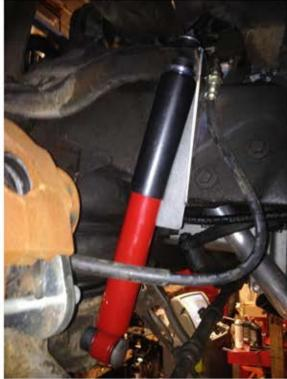
Slide the upper tower over the top of the shock stud. Let it fall into place on the frame and mock up where your relocator bracket will be welded. Tack it in place and test the shock for no binding / clearence issues - using a floor jack can help.
