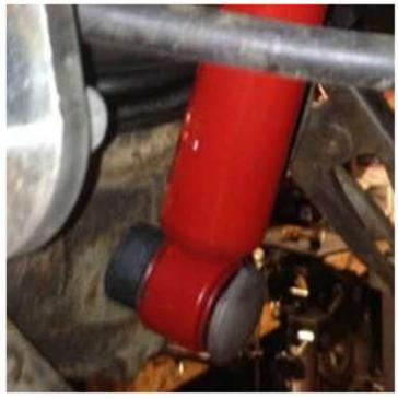
Mount the bottom eyelet of the shock through the shock stud to the lower arm.
