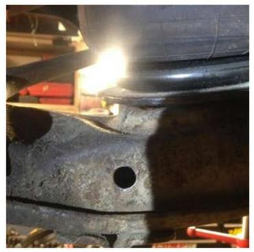
With air out of bags, fully compress the A Arm. Hold up one compressed shock and one fully extended to mock up where your hole and shock tower will land. Make sure you have clearance and no binding issues then drill a hole for the shock stud.
