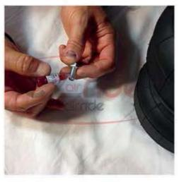
Dab some EZ Tite around the 3/8" bolts to ensure a tight fit when mounting brackets to the air bags.
