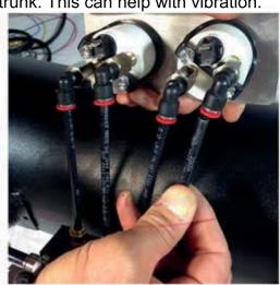
Note: Each number on the manifold will correspond to your desired corner of the vehicle.
