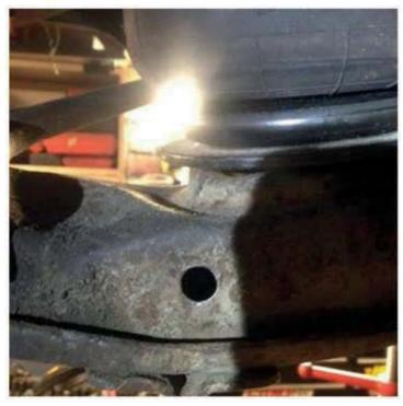
With air out of bags, fully compress the A Arm. Hold up one compressed shock and one fully extended to mock up where your hole and shock tower will land. Make sure you have clearance and no binding issues then drill a hole for the
