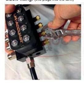
Make sure each fitting is nice and tight. EZ Tite will help to prevent leaks and ensure a tight seal.
