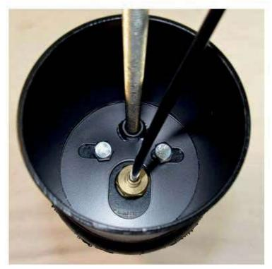
Screw the supplied all thread into the bracket. Run air line from the appropriate valve going through the shock tower and into the bag. Slide the cup into the front-upper spring pocket. Insert all thread through the shock tower and mount it in place using the supplied washer and nut. **Note: offset disk will face the wheel.**
