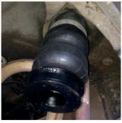
Install bottom bagel bracket to the air bage
