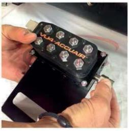
First, using EZ Tite, thread the 1/4" to 1/2" fittings into the Intake port on 2 strips of 1/2" air line 2.5" in each side of the Accuair manifold.
