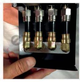
Adjust each elbow fitting so they all face through the the manifold bracket. This allows for easier and cleaner plumbing.
