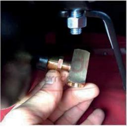
Thread the Tee into the side of the air tank.
