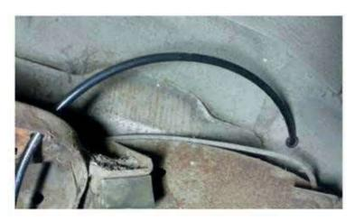
You can use a pre-existing hole in your upper spring mount to run your air line throught. Next, plumb the air line into you bag and mount the air bag and upper bracket using the suplied all thread and nut.
