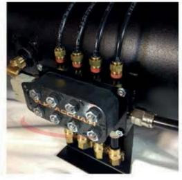
Next, run 1/4" air line from each fitting at the top of your manifold to the back of each gauge.
