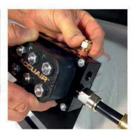
On the bottom side of the manifold Next, thread in the (4) 1/4" fittings into the top of your manifold. These will plug into your gauges. They will monitor air pressure for each bag.
