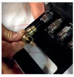
Use the (4) 1/2" elbow fittings and connect the strips of air line to the 1/4"x1/2" fittings on the bottom of the manifold.
