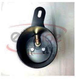
Bolt the top cup to the air bag and insert your 90 degree swivel fitting.
