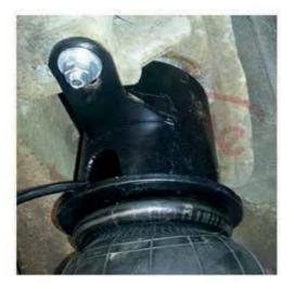
Slide the cup into the upper spring pocket, then bolt the ear to the factory bump stop mount.
