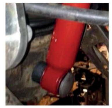
Mount the bottom eyelet of the shock through the shock stud to the lower arm.
