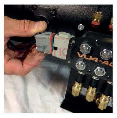
Plug the wire harness for your switchbox into the side of the Accuair manifold.
