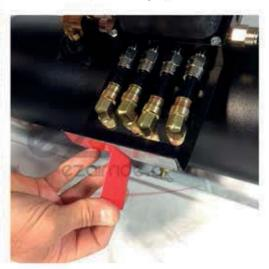
**Optional:** Peel and stick the manifold bracket to the desired spot in your trunk. This can help with vibration.
