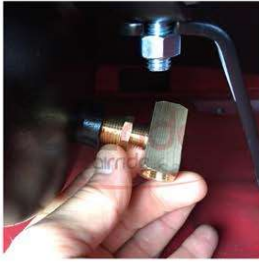
Thread the Tee into the side of the air tank.
