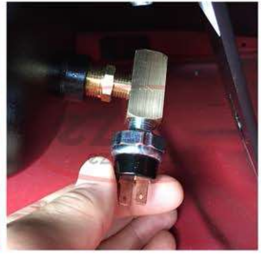
Next, thread the pressure switch into the tee. We suggest the backside Leaving the front for you Spare Air™.
