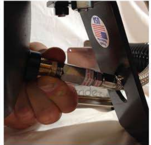
Now, plug your compressor into the side port on the air tank. Simply, through our EZ Tank Bracket hole.
