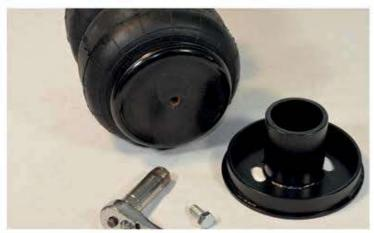
Bolt the bottom bracket to the air bag. This bracket has been designed to sit nicely in place on your lower A Arm.
