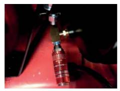
Connect the brass Tee to the side of the tank. Pressure switch (not shown) plugs into the back side and the quick connect plugs into the front.
