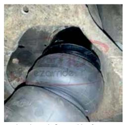
High side with flanged lip faces outward (toward the wheel). Once bag is bolted and fitting is secure, bolt all thread through the shock tower.
