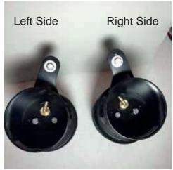
Bolt the top cup to the air bag and insert your 90 degree swivel fitting.
