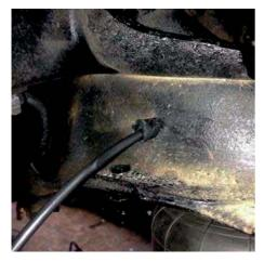
Be sure to feed enough air line through your spring pocket to easily feed into the air bag as you bolt it up
