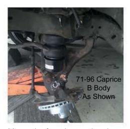
Mount the front-bottom bracket to the air bag and let it sit in the lower spring pocket.
