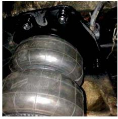
Plumb the air line into the bag fitting before bolting the assembled bag/bracket to the crossmember.
