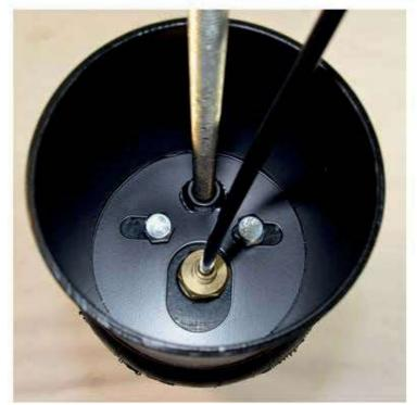
Screw the supplied all thread into the bracket. Run air line from the appropriate valve going through the shock tower and into the bag. Slide the cup into the front-upper spring pocket. Insert all thread through the shock tower and mount it in place using the supplied washer and nut. **Note: offset disk will face the wheel.**
