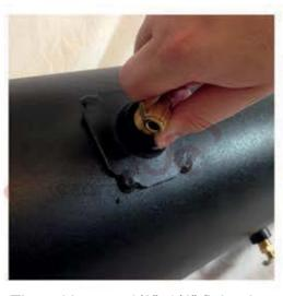
Thread in your 1/2"x1/4" fitting into one of the ports on the front of your using the supplied fitting and air tank. This fitting will supply air to tighten with a Hex Key. You will your paddle valves.
