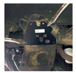
Once the coil spring has been removed use the front upper mounting plate as a template for drilling the 4 perameter holes on the upper crossmember.
