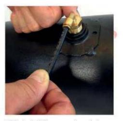
This tank fitting supplies air to the control panel.
