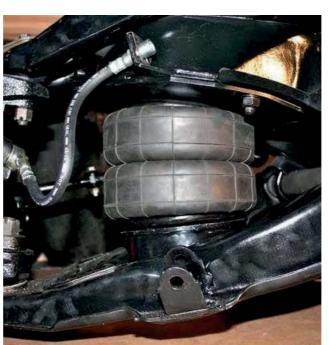
Once the mounting plate has been safely bolted in place the lower cup will sit in the factory lower A Arm.
