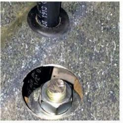
Pull out the all thread and trim it. Run your air line from the bag up through the floor board and then tighten the nut with a socket from your trunk.
