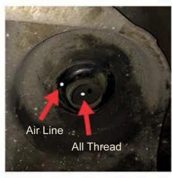
Remove your rear coil springs. Hold upper bracket in place and mark hole for air line and all thread.
