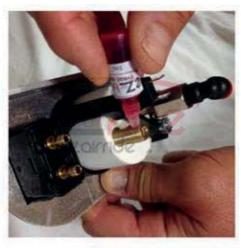
Use EZ Tite to secure the Red Head fittings on the back of the air gauge.
