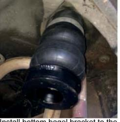
Install bottom bagel bracket to the air bag.
