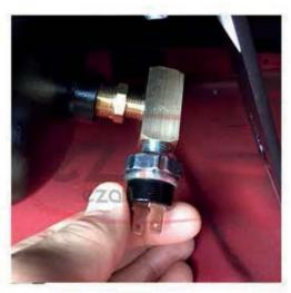
Next, thread the pressure switch into the tee. We sugest the backside Leaving the front for you Spare Air™.
