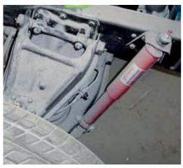
63-72 C10s have to be the coolest and easiest of them all to install air ride. It is the only GM vehicle where the shock is mounted on the outside of the coil spring, therefore no relocating.
