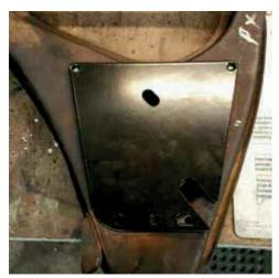
Set the bottom plate on the lower A Arm and use it as a template to pre-drill bolt holes.
