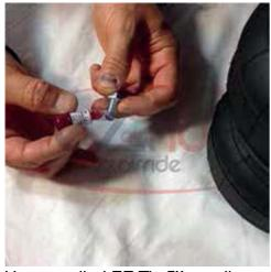
Use supplied EZ Tite<sup>™</sup> on all mounting hardware to ensure a tight fit when mounting brackets to the air bags.
