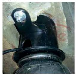
Slide the cup into the upper spring pocket, then bolt the ear to the factory bump stop mount. Note: there is a left and right hand side upper rear bracket.
