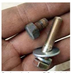
Replace the factory E-Brake bolt with the fine thread bolt supplied in your new EZ Air Ride kit.
