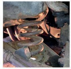
Once your vehicle is safe and secure, begin by removing the factory coil springs. To avoid possible clearance issues, your factory bump stop may
