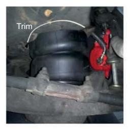
Bear in mind - when the bag is inflated, most vehicles will require you to trim the upper-outer spring pocket only. Cut a rainbow shape like the picture shown above.
