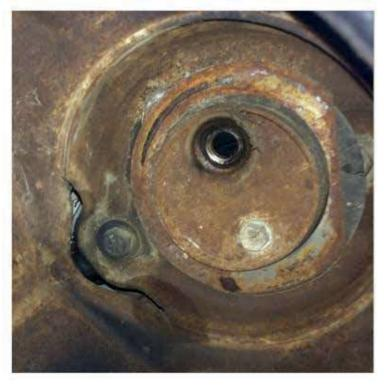
First, remove front coil springs. Bolt the front-top cup to the air bag and thread in the straight fitting.
