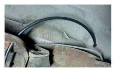
You can use a pre-existing hole in your upper spring mount to run your air line throught. Next, plumb the air line into you bag and mount the air bag and upper bracket using the suplied all thread and nut.
