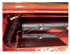
When finished replace the schrader valve with the supplied coil hose and air chuck. You now have onboard air!
