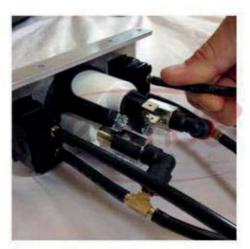
Now, plug 2 more strips of air line into the delivery barbs on the back of the gauge labeled "SUP." These barbs will "supply" air to your bags.
