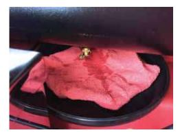
Depending on your climate, how much you use you air ride system, and the overall humidity will determine how often you should drain your tank. Simply, use a frisbee and the complimentary shop towel to catch any water or debris. With that being said, you may want to start off by draining it once per month. Slowly open the drain cock, catch any moisture with your new shop towel, then tighten your drain cock. Your new Spare Air<sup>™</sup> kit will make filling your tank back up a breeze!
