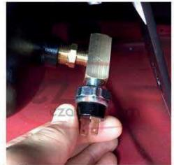
Next, thread the pressure switch into the tee. We sugest the backside Leaving the front for you Spare Air™.
