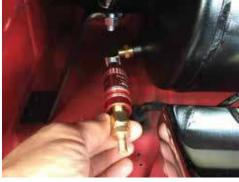
Simply, push the assembled schrader valve into the quick connect.
