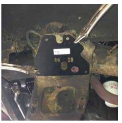
Once the coil spring has been removed use the front upper mounting plate as a template for drilling the 4 perameter holes on the upper crossmember.
