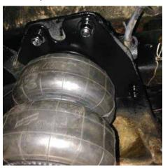
Plumb the air line into the bag fitting before bolting the assembled bag/bracket to the crossmember.
