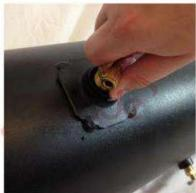
Thread in your 1/2"x1/4" fitting into one of the ports on the front of your air tank. This fitting will supply air to your paddle valves. On the neighboring port, plug it off using the supplied fitting and tighten with a Hex Key. You will not need to use this port.
