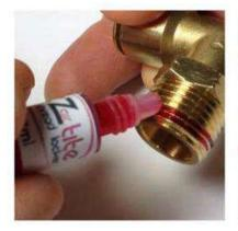
First, put a little bit of EZ Tite around the thread of the fitting you are installing. This will keep air from leaking and ensure a tight seal.
