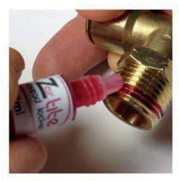
First, put a little bit of EZ Tite around the thread of the fitting you are installing. This will keep air from leaking and ensure a tight seal.
