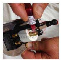
Use EZ Tite to secure the Red Head fittings on the back of the air gauge.
