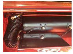
When finished replace the schrader valve with the supplied coil hose and air chuck. You now have onboard air!
