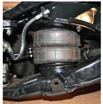
Once the mounting plate has been safely bolted in place the lower cup will sit in the factory lower A Arm.
