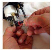
Next, plug the 1" air line strip from the Tee to the Red Head gauge fitting.
