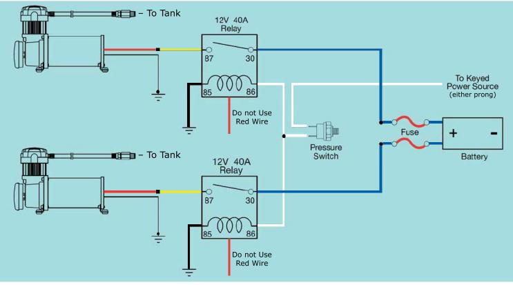
Ground Wire– The ground lead on the compressor should not be extended (if possible). Always connect ground leads directly to the chassis (frame) of the vehicle. Any other grounding method may result in amp spikes that can damage the compressor motor by causing sporadic and undesired operation.
