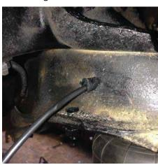
Be sure to feed enough air line through your spring pocket to easily feed into the air bag as you bolt it up
