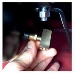
Thread the Tee into the side of the air tank.
