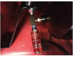
Connect the brass Tee to the side of the tank. Pressure switch (not shown) plugs into the back side and the quick connect plugs into the front.
