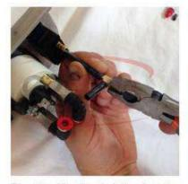
Plug the 2" strip of air line into the delivery barb on the back of the paddle. This will be labeled "DEL."
