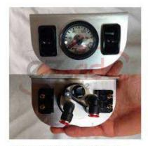
This is your new EZ Air Ride Classic gauge control panel. The dual needle gauge will monitor the air pressure in your air bags. The left paddle controls the front and the right controls the rear.
