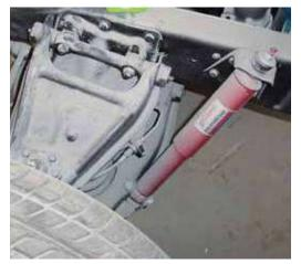
63-72 C10s have to be the coolest and easiest of them all to install air ride. It is the only GM vehicle where the shock is mounted on the outside of the coil spring, therefore no relocating.
