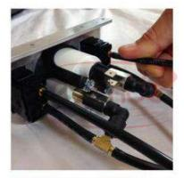
Now, plug 2 more strips of air line into the delivery barbs on the back of the gauge labeled "SUP." These barbs will "supply" air to your bags.
