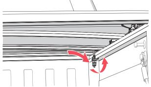
Hand tighten the clamps to hold the cover in position.
