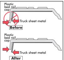
Measure and trim the plastic high enough to expose the truck sheet metal, and wide enough to accommodate the clamp.
