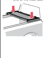
the truck bed for proper front (cab) / rear (tailgate) alignment. When positioned front and back, the tailgate seal should contact the tailgate with the first two fins.
