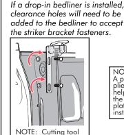
Insert the nut plate down through the stake pocket opening and align with the 5/16" striker bracket bolts.
