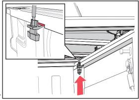
Slide the cab clamps over to the truck bed rail. Hook the clamp jaw under the truck bed rail.
