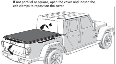
Close the tailgate and unfold the cover. Check that the cover
