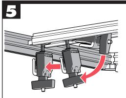
The front (cab) clamp stows in the cover rail. Rotate the clamp down and slide it towards the bed rail.
