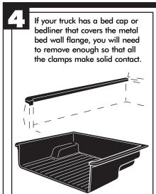
For bed caps, trim only enough of the bed cap edge so the rear (tailgate) clamp contacts the bottom of the metal flange.
