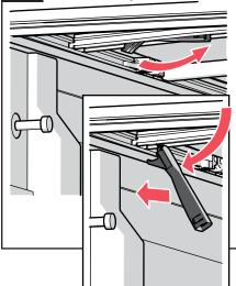
The clamps should be slid as far over to the truck bed rail as possible.
