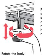
of the clamp up or down to match it's position with the bed rail flange.
