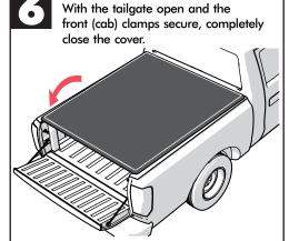
The rear (tailgate) clamps are stowed in the cover rail, rotate the clamp down and slide it to the truck bed rail.
