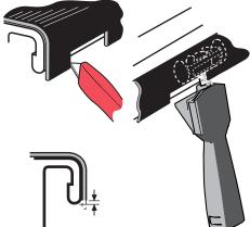
For bed liners that cover the metal flange, trim a minimum of 100 mm or 4" of the liner wall so the clamps contact the bottom
