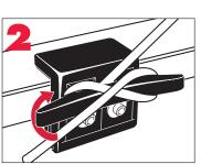
All weight bearing rope or hooks MUST be in the CENTER hole as shown below.
