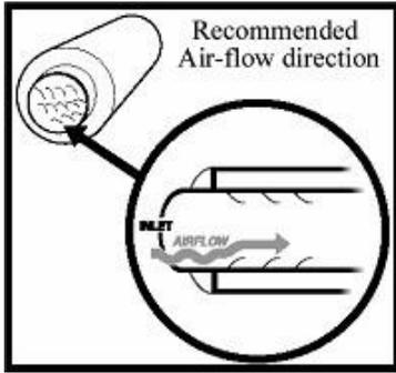
3. Install the **Muffler** over the **Extension Pipe**. Refer to the figure on the left for correct **Muffler** orientation.
