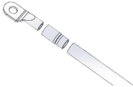
Figure 2-7 Copper terminal, heat shrink tube and copper wire.
