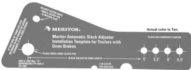
TP-4787 ASA template for trailers with drum brakes. NOTE: Trailer must always use 1.38" spacing!
